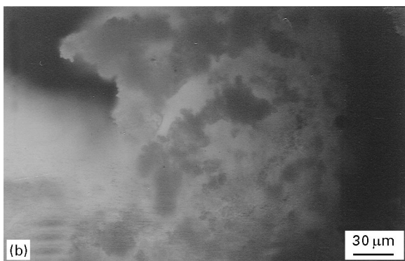
Figure 2 Polarized light optical micrographs of a CHI-PSS ([SS]/[CHI] = 6) complex (a) and of a corresponding "mixture" (b).
